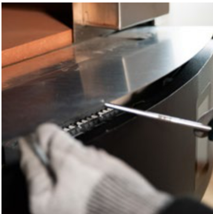
3. Lift the steel guard using a screwdriver.
