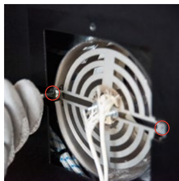
2. Unscrew the 2 fixing screws on the locking grid and remove the lamp to be replaced.
